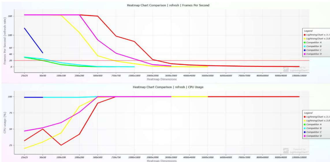
Visualization of refreshing heat map benchmark results. X axis = heat map data set size, Upper Y axis = Refresh rate (higher value is better), Lower Y axis = CPU usage (lower value is better).
