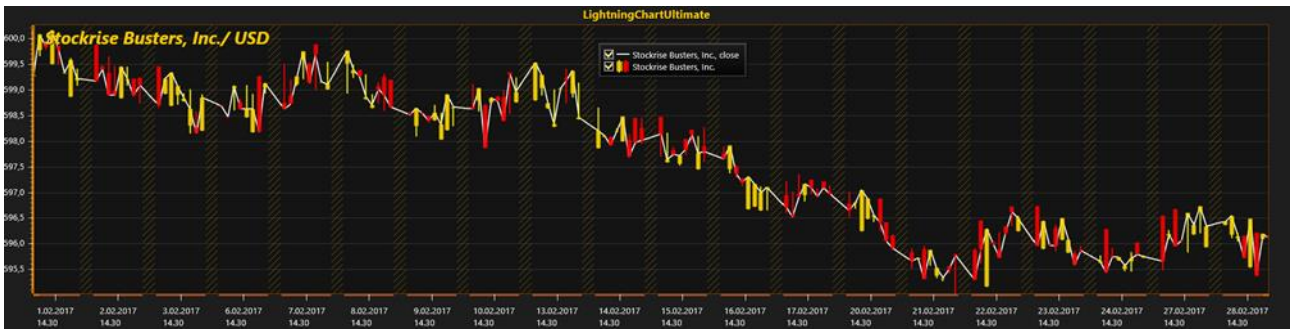
图 6-36. 在无活动交易时间应用 ScaleBreaks; Style = DiagonalLinesUp, Gap = 20. PointLineSeries.ContinuousOverScaleBreak = True.
