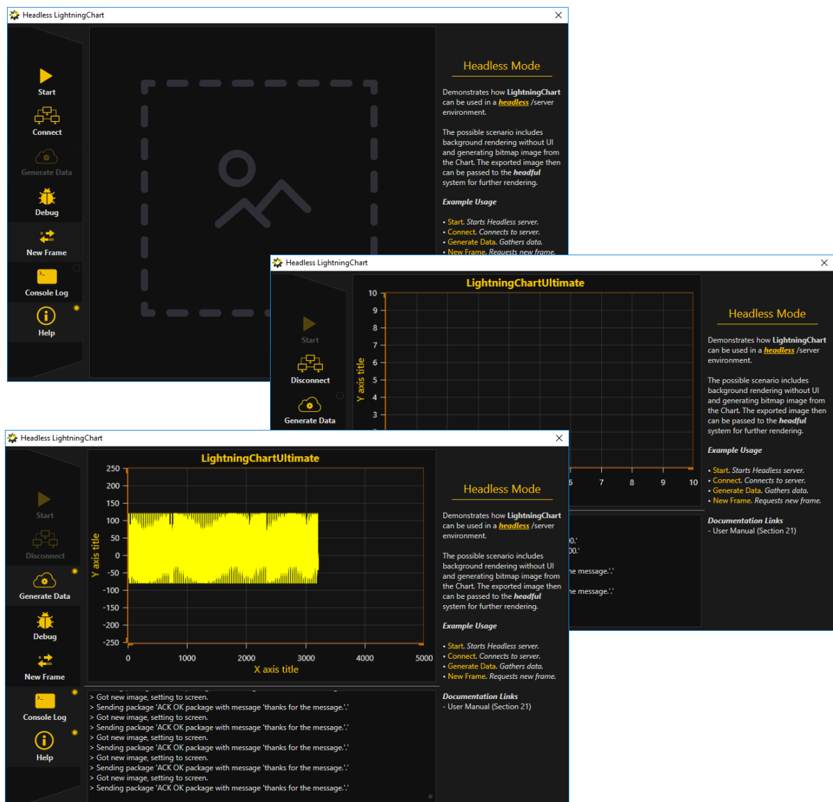
Figure 25-2. WPF client app. After Start, Connect and Generate Data, it shows continuously updating image stream.
