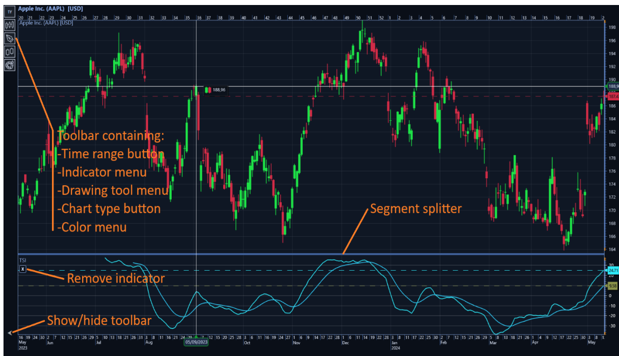
Figure 18-4. TradingChart's main user interface components, all of which can be hidden by disabling the respective property.
