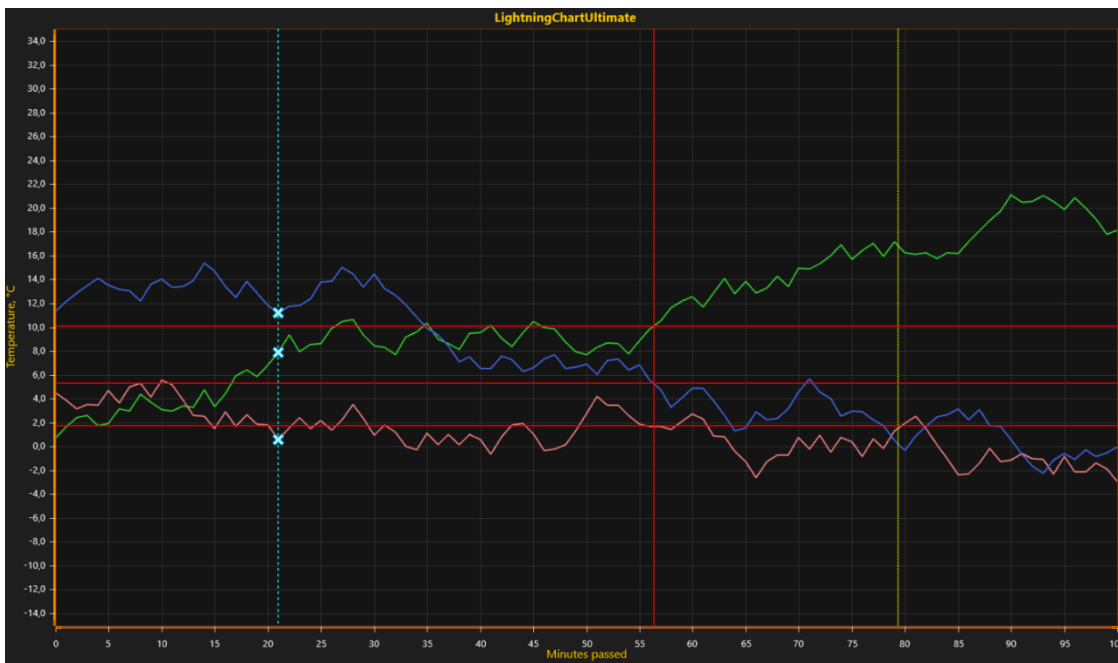
Figure 6-126. Line series cursors: Cursor on the right (cyan line and crosses), Style PointTracking , vertical point tracking cursor. Cursor in the center (red lines), Style HairCrossTracking , hair-cross tracking cursor (horizontal lines are same color as LineSeriesCursor itself). Cursor on the left (yellow line), Style VerticalNoTracking , vertical full-length cursor without tracking.
